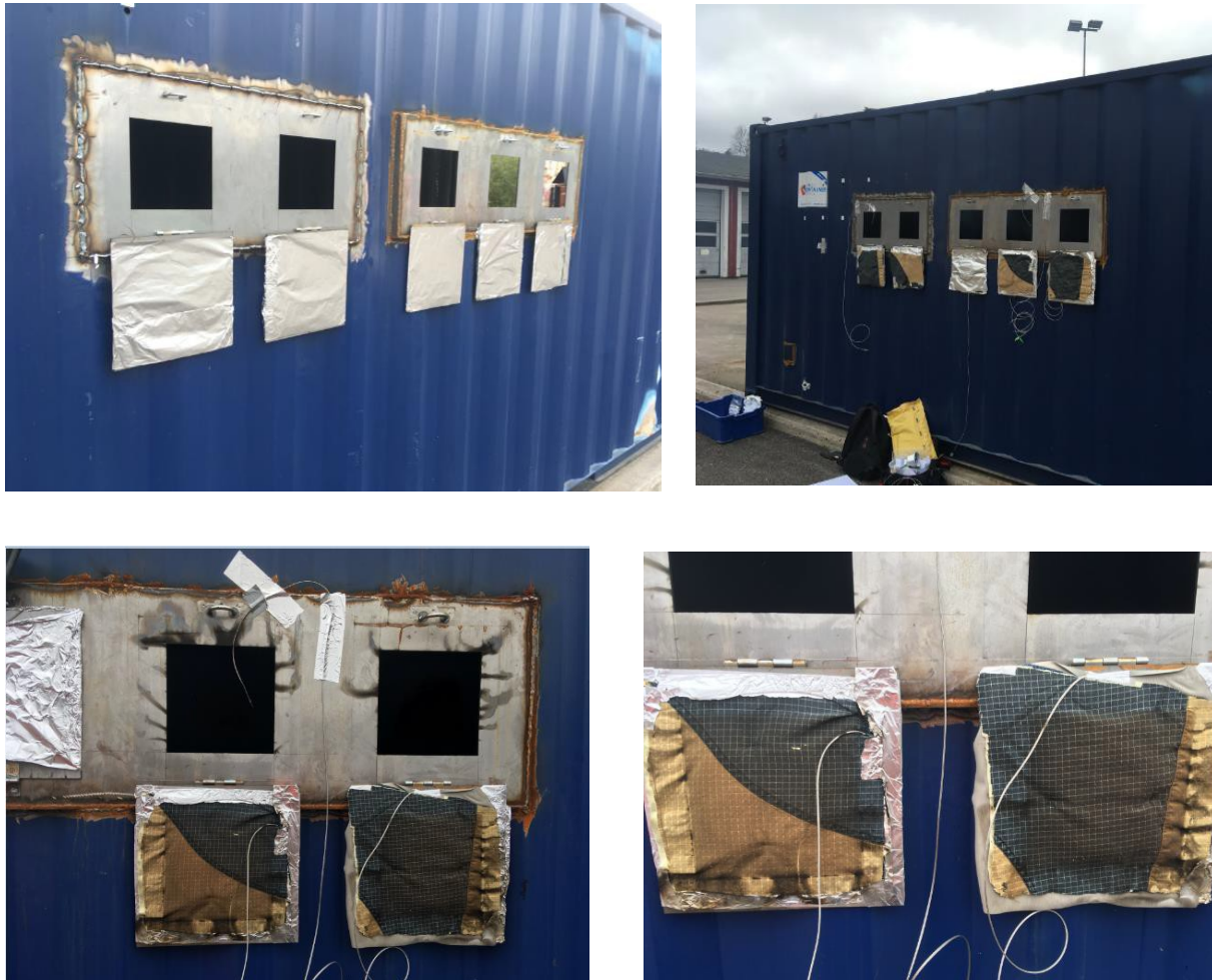
Figure B1.3 The test rig seen from outside. The left top photo shows the hatches before the material samples were applied. The top right photo shows the material samples when they have been applied for the test. The two lower photos show the material samples after exposure of fire smoke.
