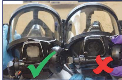
**Figure 32:** BA mask filters after and before the cleaning
