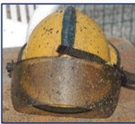
**Figure 12:** An example of surface contamination
