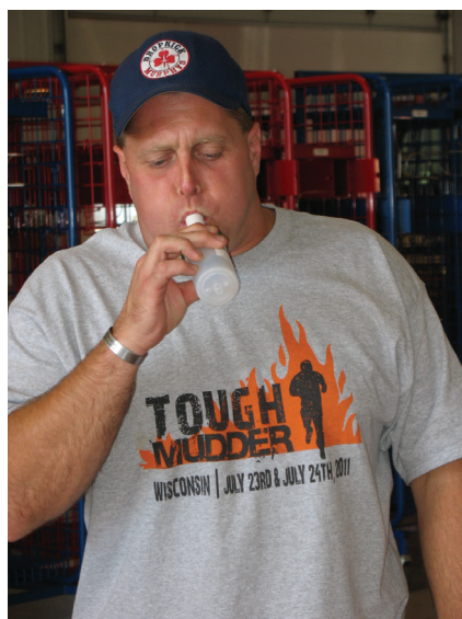
Figure 5. Participant exhaling into the Bio-VOC sampler. Photo by NIOSH.
